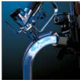
**Self-cleaning in 7 minutes** thanks to QuickClean, the suction tube with a gun connection. Pull off the gun, lock it and the SF 31 immediately starts to clean itself automatically, allowing you to take care of more important things.
