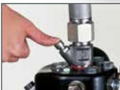
The inlet valve push-button ensures a high level of **operational safety**. Press it once with your thumb and the valve is free.
