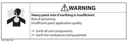
Any material containers and the unit must be connected by a potential equalisation (earth) cable.
