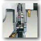
The new practical, **self-adjusting packings** lead to less wear and are easy to change. They have a service life up to 50% longer than the current packings which means significantly lower maintenance costs.
