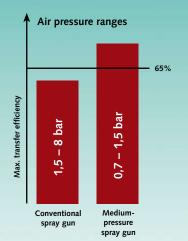
A transfer efficiency in excess of 65% was measured for the new WALTHER PILOT medium-pressure models.
